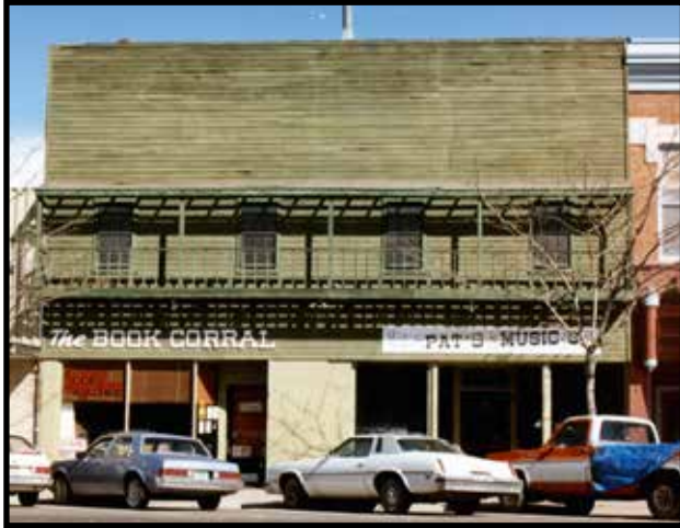
621 - 623 Main Street shown on the left with inappropriate window placement and façade. The faux façade was removed in 2003 exposing the original tall windows, storefront cornice, transom windows, and brick façade.
