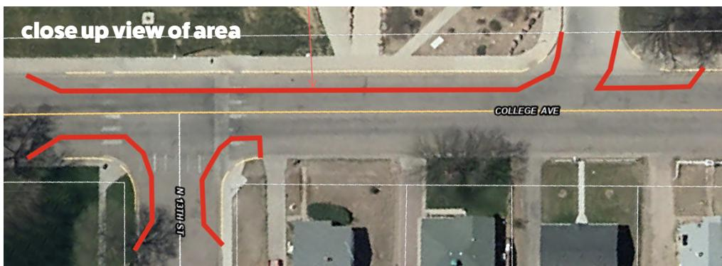
6-foot wide concrete blocks and 48-inch tall green delineators will be used for the temporary traffic calming installation in the areas outlined in red on the maps.
