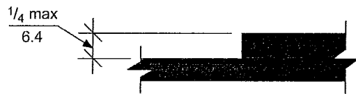
Fig. 303.2 Carpet on Floor Surfaces
